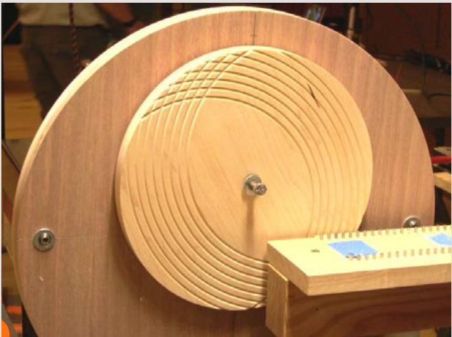
Demonstration disk after second offset 9.5" dia. demo disk 16" dia. faceplate.
