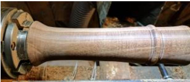
Jobillo has distinct grain and color but it is mostly in straight lines. Inclusion of the beads is appropriate for this piece of wood. The two small beads were turned with the D-Way beading tool and the large bead was turned with the skew chisel. The bottom part of the peppermill is shaped primarily with the spindle roughing gouge. French curve scrapers are useful in final shaping of the top.
