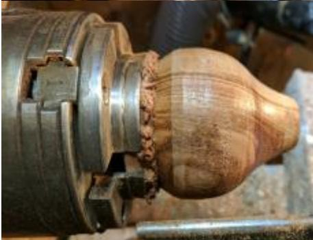
The top of the mill is shaped in the chuck, held by the tenon. The round part seen above mill can be spherical or compressed and oval, whatever you like. The tapered bottom part is to smooth the line and fit with the bottom. Extending the top down inside the throat of the mill stabilized the rotation of the grinder. Before removing from the chuck, cut the groove to hold the shaft clamp (see below).
