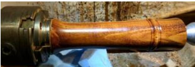
At this point, the bottom can be sanded and finished. This piece was sanded to 600 grit using walnut oil as a sanding lubricant. The piece was friction polished with fresh walnut oil and finished with three coats of Pens Plus.
