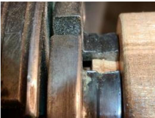
Make sure that the shape of the tenon matches the chuck jaws. This is a Nova 50 mm jaw, and therefore has a dovetail. Size the tenon to allow the jaws to close almost completely to get the strongest grip on the wood.
