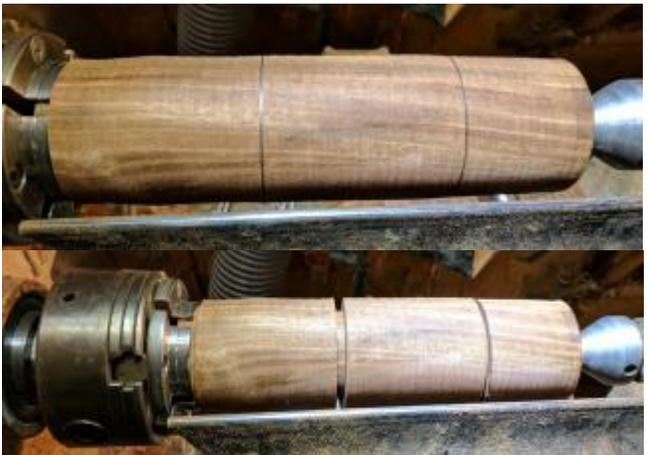
To turn the bottom part of the mill, layout the approximate location of important features. Here, the narrowest point of the mill as well as the location of the rings at the bottom have been marked.
