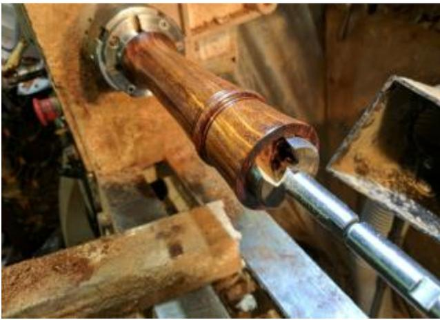
The outside of the bottom is finished and now the milling of the interior begins. I use the Colt Maxicut Rotastop forstner bits. These are by far the sharpest and truest running forstner bits. Also, the Rotastop feature makes extensions very easy to use. A 1.75" wide, 0.75" deep relief is drilled into the bottom of the peppermill. This allows for the adjustment nut on the bottom of the Crush Grind mechanism. There are three drilling steps. The first one is the 1.75 by 0.75" opening in the base.
