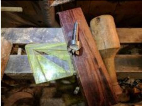
The process begins with a blank, about 3 x 3 x 12". About any wood will do but harder wood, like this piece of jobillo, takes detail very well and mills easily.
