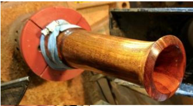
The trumpet needs to be big enough to hold the tapered top section, which is fitted to it during shaping. The trumpet is sanded to 600 grit using walnut oil sanding we were good and finished with three coats of Pens Plus.
