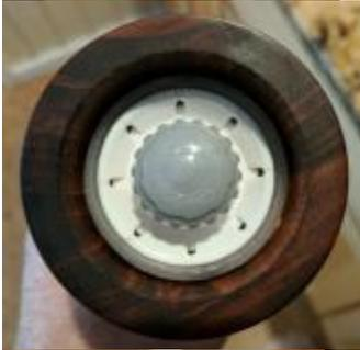
This is the view from the bottom with the grinder in place. The gray nut determines the texture of the ground material. It can be loosened or tightened to control fine and coarse grinding.
