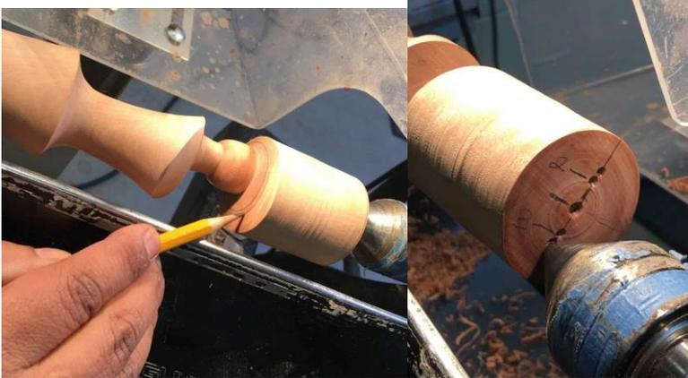
6. Top of hat: Loosen the chuck and shift the cone center back to center point #3. The top of the hat must align with the lower part of the head which is under the hat brim. The
