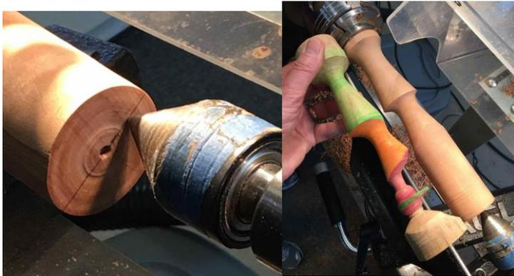
4. Head and Neck: Loosen the chuck and shift the cone center  $1/2$ " to the opposite side of the center hole. Retighten. Check the wood being removed. If not enough or too much, make a minor change in the location of the cone center. This will be cone center point #3. Cut in to form the neck to the desired diameter. Then cut the head to the desired diameter. Keep in mind the proper proportions of the human body for the
