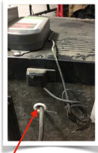
*Run the powercord from the outside back through the existing hole with the white rubber grommet.*
