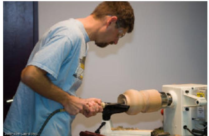
Trent's Vessel of Illusion sample and depth drilling using a gun drill and compressed air. Photo: Andy Johnson-Laird
