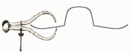
These calipers with matching legs are used to measure walls to a set size. You can adjust the amount of opening at the tip by turning the adjusting screw. This is very useful when the same setting on the calipers can access the entire object. When turning a hat these calipers are the tools of choice. When the object gets bigger your calipers must get bigger also, but the bigger ones are very expensive and hard to find.
